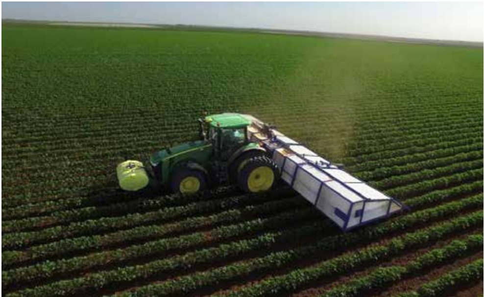
Figure 2. Autonomous machine performing spraying operation to harmful herbs
